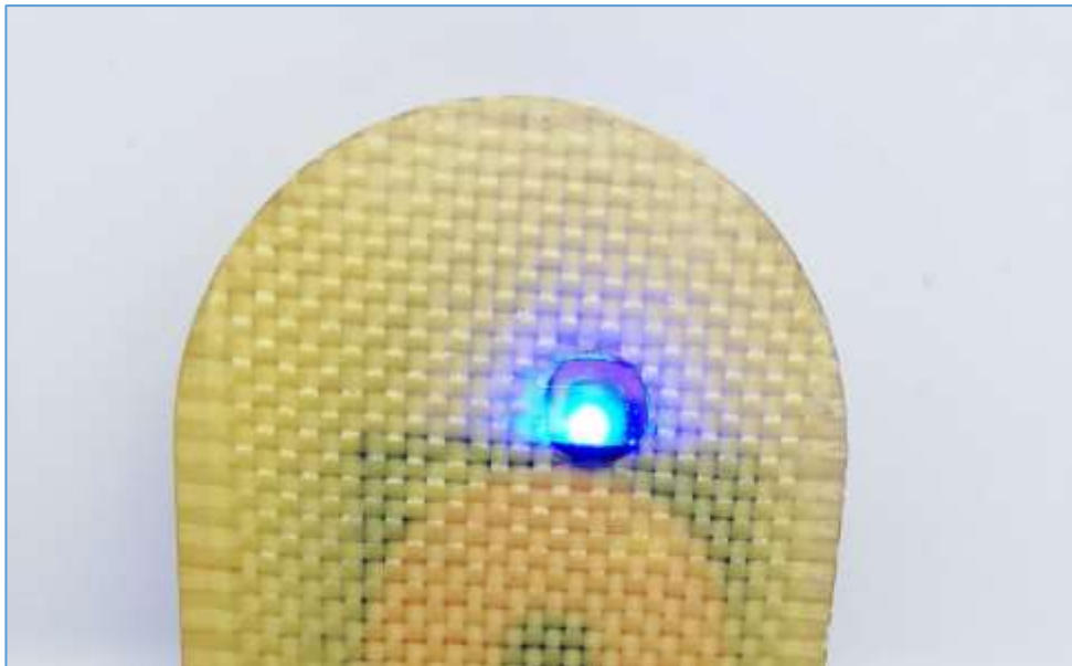
Electronic module of XSole PTI insoles embeds a LED
